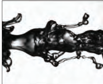
Ligament Mediated Drop Formation, Ph. Marmottant and E. Villermaux, LEGI, Grenoble and IRPHE, Marseille
